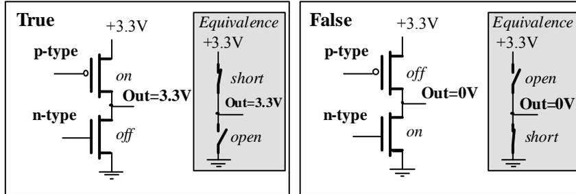
Logic high is 3.3V, logic low is 0V. Assuming a fixed resistance  $R$ , the +5V logic has a power of  $5V \cdot 5V/R$ , which equals  $25/R$ . The +3.3V logic has a power of  $3.3V \cdot 3.3V/R$ , which equals  $11/R$ . This is a reduction in power by a factor of  $11/25 = 44\%$ .
